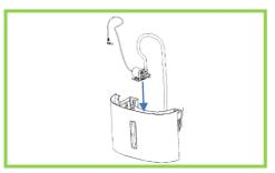
**Step 3:** Secure the pump in the space directly beneath the handle using the suckers attached.
