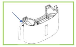
**Step 4:** Put the water tank lid back in place, allowing the hose and power lead to exit the water tank in the gap on the left-hand side.
