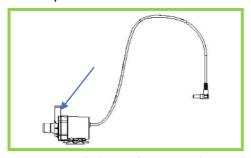
**Step 1:** Connect the hose to the pump via the vertical outlet.
