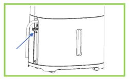
**Step 5:** Push the water tank back into the dehumidifier and remove the small rubber cover in the left-hand side recess. Insert the power connector.
