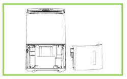
**Step 2:** Remove the water tank from the dehumidifier, lift the water tank handle and remove the water tank lid.
