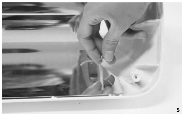
5. APPLY THE SPARE HEAT-ELASTIC CAPS TO REPLACE THOSE WHICH HAVE BEEN REMOVED. STRIP THE CORDS (5-6 mm). APPLY THE NEW SPARE FASTONS AND PRESS THEM ONTO THE STRIPPED PORTION OF THE CORDS. DO NOT TOUCH THE BULB WITH YOUR BARE HANDS.
