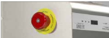
Fig. 2.5.2.A: Emergency off switch
