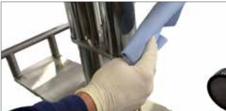
Fig. 8.3.2.A: Remove abrasive residue from the lifting column
