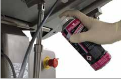
Fig. 8.3.1.A: Apply spray to the cylinders
