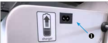
Fig. 3.6.3.A: Connection charging cable (1)
