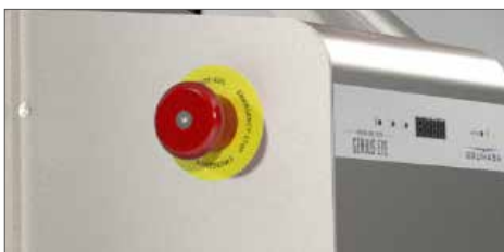
Fig. 6.3.A: Emergency off switch
