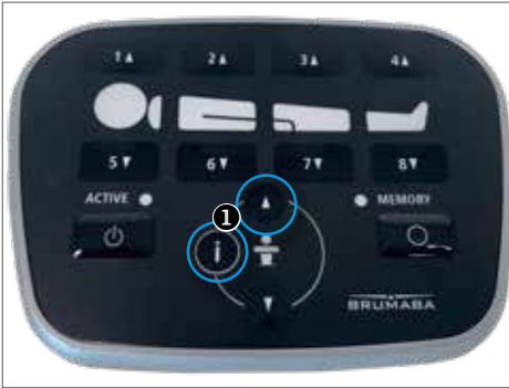
Fig. 6.10.A: Key combination for showing the battery voltage (1)
